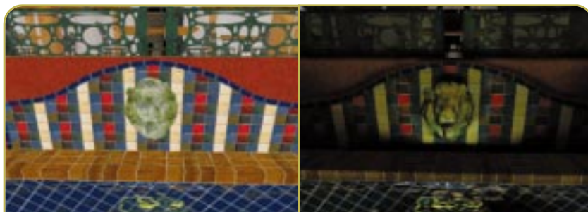
FIGURES 3A AND 3B. 3A is a scene lit without shadow maps, 3B has shadow maps applied, both on Nvidia TNT.
