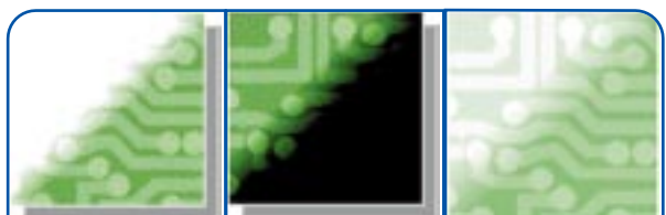
FIGURES 5, 6 and 8. Additive blending result, subtractive blending, and the result of additive blending without overflow.
