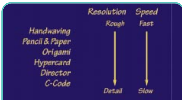
FIGURE 6. Prototyping tools that cannot represent a lot of detail are generally faster than those that can more accurately represent the final product.
