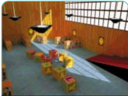
FIGURE 4. The AnyWorld engine. The walls and floor are tiled with smaller textures while large light maps add highly detailed lighting to the scene.
