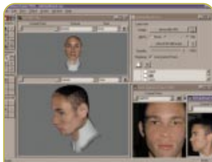
Using SurfaceSuite Pro's control-point-based mapping system to map a photo onto a 3D model.
