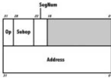
FIGURE 5. Our command structure is similar to the structure of standard N64 microcode commands. We use this structure for all of our commands.
