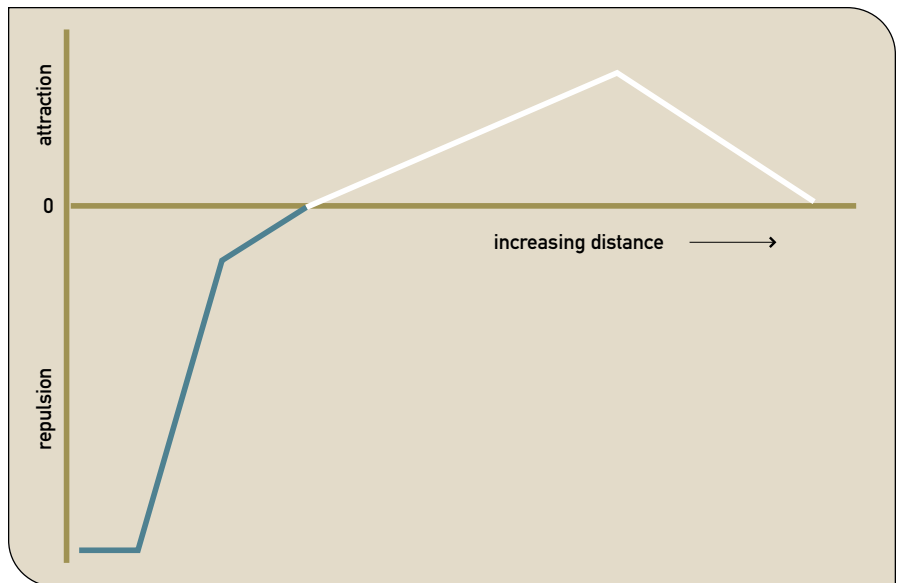
FIGURE 4. The force function used for molecule vs. molecule interactions.
