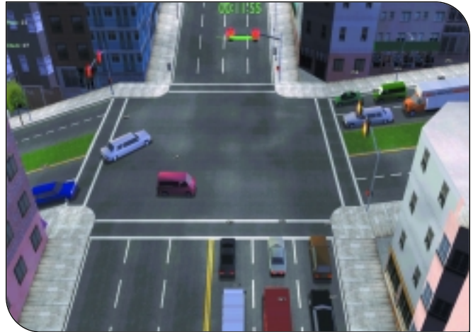
FIGURE 2. In this case, the TrafficLight class is set to red for some vehicles, which stop and wait. The other vehicles with green/yellow lights get permission to cross the intersection. The vehicle crossing in the left lane decides to turn left, while the vehicle in the right lane goes straight.
