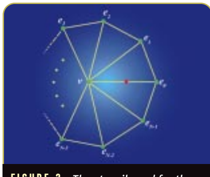
FIGURE 2. The stencil used for the extraordinary case of the modified butterfly scheme.
