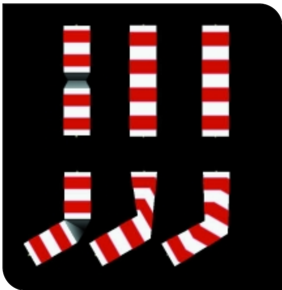
FIGURE 6 (top). Three different joint attachments in wireframe. The joint on the left is two separate pieces of geometry, in the center is a joint built with clusters of vertices, and the joint on the right was built with weighted vertices.
