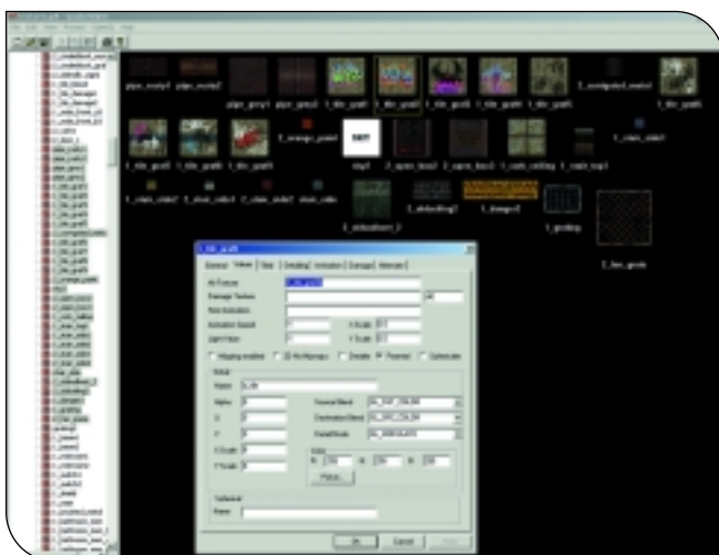
LEFT. Raven developed QuakeHelper to manage more than 5,000 unique world textures with a visual means to assign properties to them.
