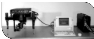
FIGURE 7 (above). SOC-250 in situ bidirectional reflectometer. FIGURE 8 (right). SOC-200 laboratory bidirectional reflectometer.
