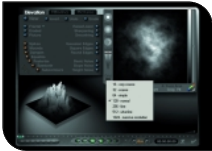
FIGURE 3. Mesh resolution in Bryce 4 is based upon grayscale image resolution.
