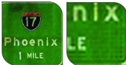
FIGURE 1A (left). Original image of a road sign. FIGURE 1B (right). A close-up of the corner after mipmapping via the discrete Fourier transform. Note the unwanted bands of color ("ringing").
