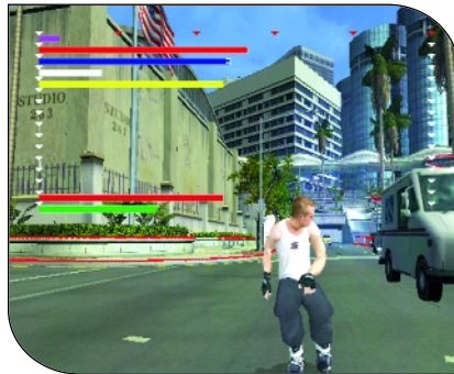
Profiling performance of the Playstation 2 version of AGGRESSIVE INLINE. Full horizontal deflection indicates dropping to 30 fps. The red bar at the top is VU, the blue bar CPU, the green bar at the bottom is game code CPU usage. The red lines on geometry are edges tagged for grinding.
