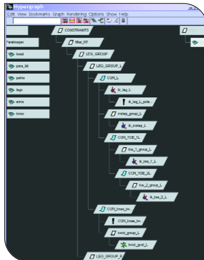
FIGURE 5. The leg constraint hierarchy viewed in the Hypergraph, showing connections between the IK handles, locator set, and NURBS constraint objects.
