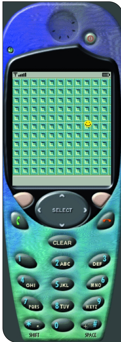
THE MIDP 2.0 EMULATOR IN ACTION. This example is running at a glorious two frames per second with a single sprite and a simple tilebackground layer.
