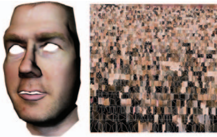
Figure 2. A perfectly authalic—and perfectly unreadable—map, generated by applying an individual planar projection to every face in a model.
