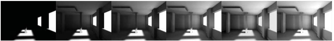
FIGURE 4 Progressive refinement—light comes in only through the window and bounces around the room, brightening it.
