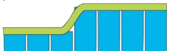
FIGURE 2 How a height map is interpolated into a shaded render: The shading information is generated by a surface wrapped over the height field of the bump map. The interpolation of the shading surface produces the beveling effect in Figure 1.
