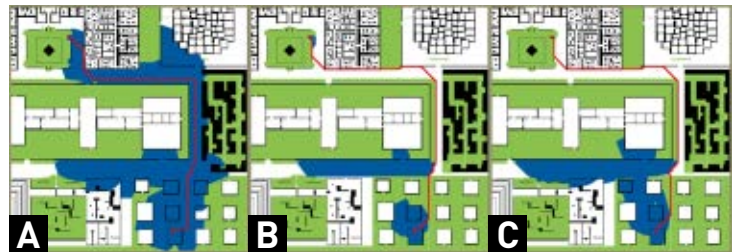
FIGURE 2 In these three pathfinding solutions to the same problem from a point near the bottom to a point at the top left, each uses the normal admissible heuristic multiplied by some constant k , and ends up expanding n nodes. Figure 2A is admissible, where k=1 and n=160,000 . Figure 2B is inadmissible, where k=2 and n=80,000 . Figure 2C is inadmissible, where k=3 and n=1,300,000 .
