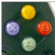
FIGURE 1 This square arrangement of buttons on the Xbox joypad is the common arrangement on current consoles.
