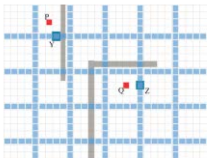
FIGURE 3 Using a fixed grid of tiles allows a non-recursive strategy for reducing precomputed storage by storing the distances between all blue tiles, such as Y and Z, as well as distances between blue tiles and nearby white tiles, such as P and Y or Q and Z.
