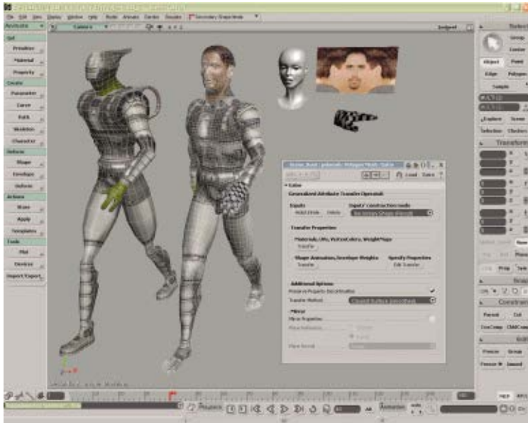
The GATOR tool, new to XSI 5, lets you transfer materials, texture UVs, vertex colors, property weight maps, envelope weights, and shape animation from one object to another.
