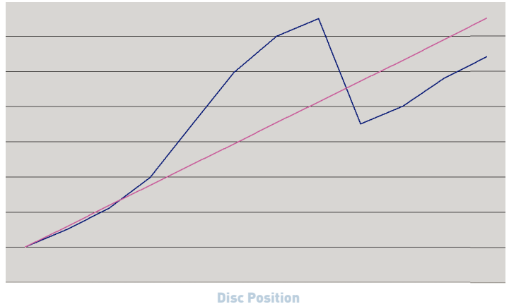
FIGURE 1 Transfer rates are expected to increase linearly as disc position changes. Real world tests prove otherwise.
