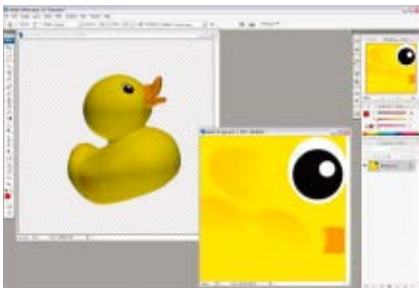
FIGURE 1 Adobe Photoshop CS3 Extended introduced direct support for Collada documents. As a result, artists can edit the textures of a 3D model and see the result from within the same tool, which makes for a big productivity boost.
