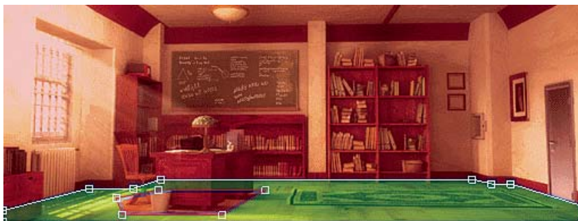
FIGURE 4 Areas where the player can walk are shown here superimposed on the background. Traversable areas are depicted in green, whereas blocked areas are shown in red. Polygon vertices are shown using white rectangles.
