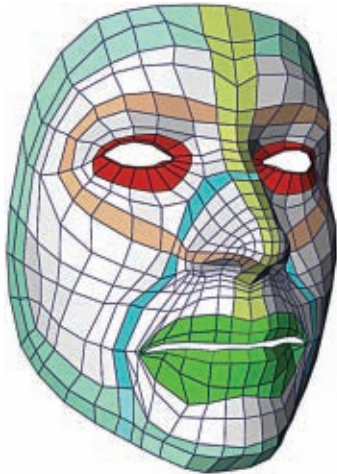
FIGURE 3 Good edge loops are essential to building up a good head-modeling workflow. This model shows a minimal set of edge loops for good facial subdivisions: the jaw line (cyan), the orbital ridges (orange), the eye sockets (red), the labio-nasal fold (blue), and the mouth (green).
