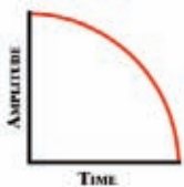
FIGURE 2 A brass instrument's decay envelope is shown.
