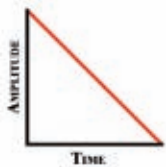
FIGURE 1 A string instrument's decay envelope is shown.
