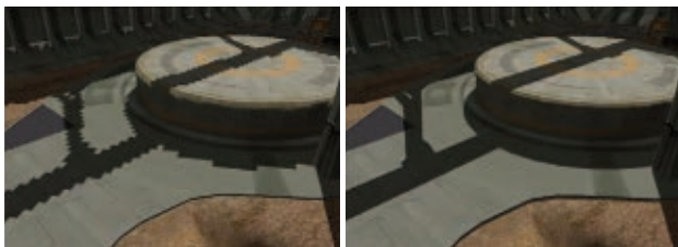
FIGURE 1 High perspective aliasing (left) vs. low perspective aliasing (right).
