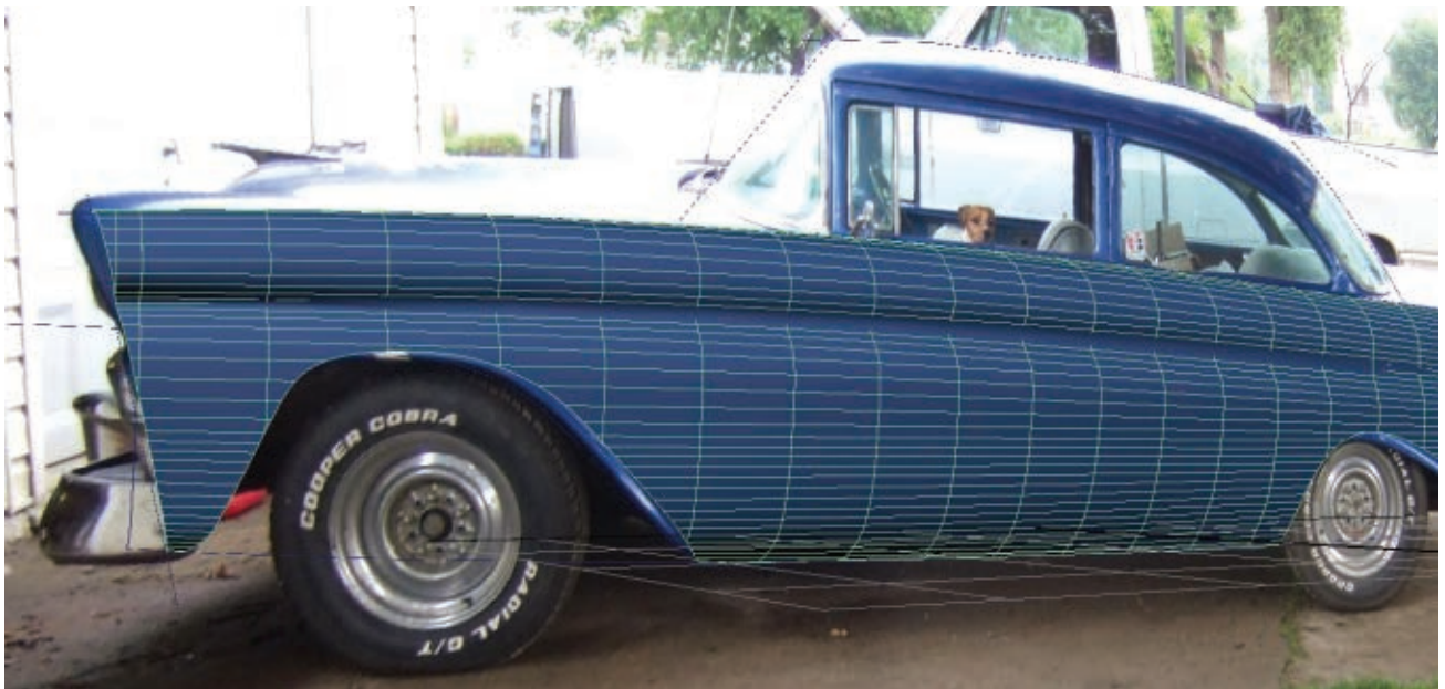
FIGURE 4: Trimming is a unique and powerful feature of NURBS modeling. This is the ability to mark out areas of a smooth surface to be discarded. It's a very powerful tool for handling tough modeling jobs where an object has continuous curvature but is divided by doors, windows, or other cutouts.
