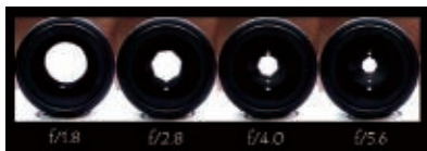
Aperture shape depending on the f-stop. We can see now where the bokeh shape is coming from!
