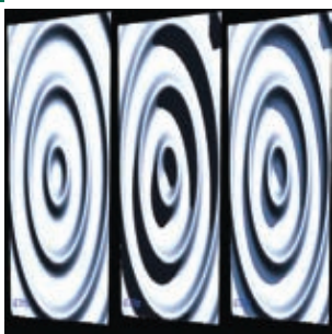
Figure 7: Left to right: Bump mapping with no self-shadows, darker self-shadows, and lighter self-shadows.
