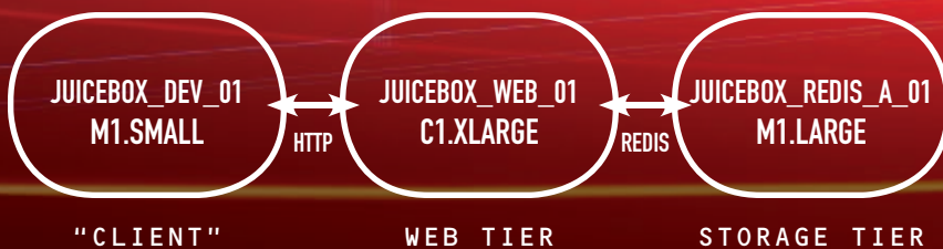
FIGURE 1: The three different dedicated AWS instances we used to generate a load for our web framework benchmarks.
