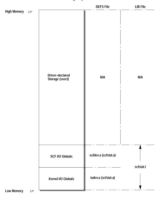
Figure 3.1 SCF Static Storage Layout
