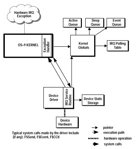
Figure 1.5 I/O System Layout for IRQ Service Routine
