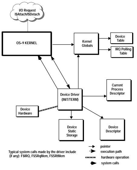
Figure 1.4 I/O System Layout for READ/WRITE/GETSTAT/SETSTAT Routines
